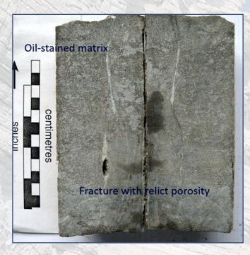
Well with water cut from oil leg in fractured reservoir: Triassic Dolomite, Middle East.
